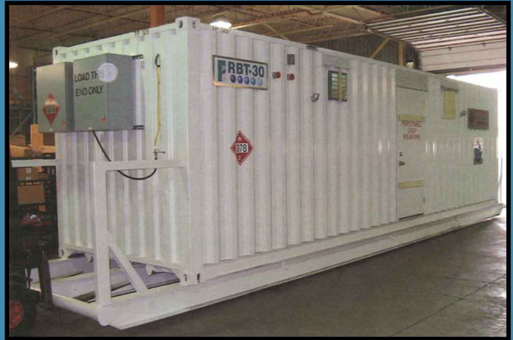
FII MicroClear™ MBR IN A 30-FOOT CONTAINER
