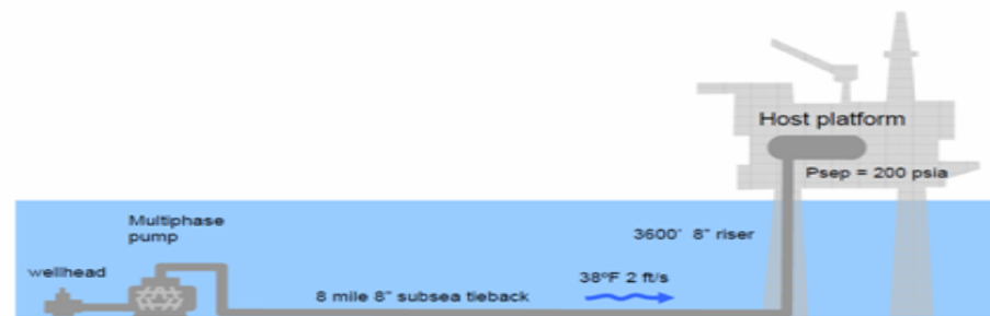
Figure 11: Schematic of Production System using subsea multiphase pump
