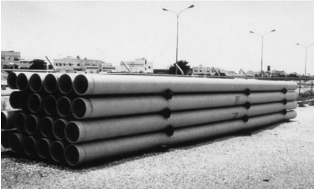
Figure 19-1. Fiberglass-reinforced pipe is frequently transported and stored as a unitized load. Courtesy of Amitech USA.
