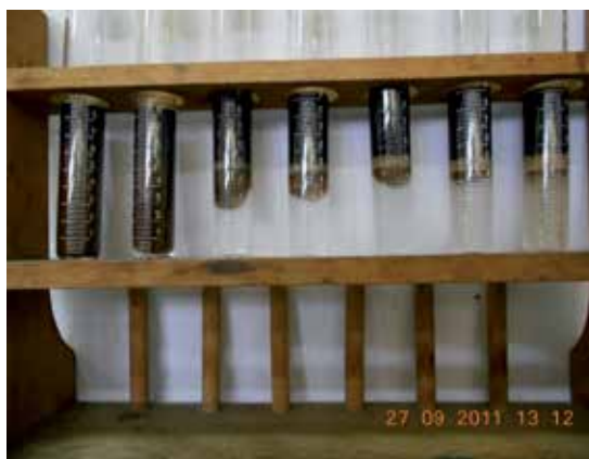
Figure 3. Stability bottle test of water-in-crude-oil emulsion (Silva, 2012).
