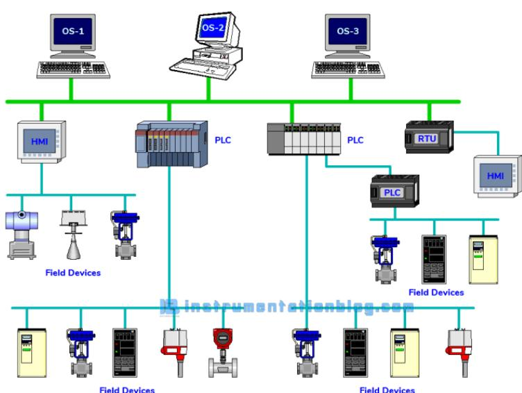
system. The HMI displays real-time data and allows operators to control and monitor the processes.
