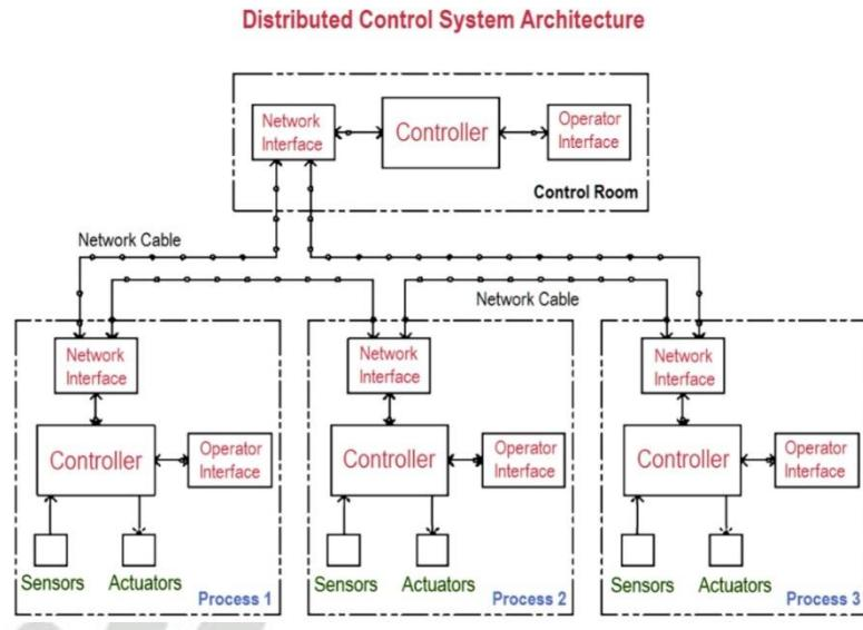
The operator interface provides the operators with a graphical display of the process, allowing them to monitor the process in real-time. The interface also enables the operators to control the process by changing setpoints and adjusting control parameters.
