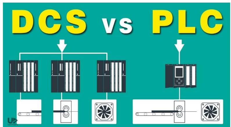
**Communication:** PLCs communicate with other devices over a limited range of communication protocols, while DCSs can communicate over a broader range of protocols.
