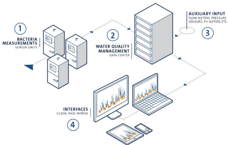
Figure 9.4 An overall illustration of a BACMON solution. A number of Sensor Units (1) send their results to a Water Quality Management server (2) into which other inputs in principle could be given (3) and from there extracted to different Interfaces (4).
