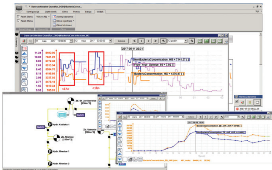
Figure 9.6 An example of integration of BACMON data directly into the SCADA system of a water utility. They use a number of different views/windows to operate their entire network and some are shown here, to illustrate how BACMON is integrated deeply into the individual views of the entire system and not just as a stand-alone window. Bottom left is a stylized map of their network and the sensor unit locations are visible as icons in this. The three windows upper right are different views used to manage the network where BACMON readings are integrated. In this way comparisons can be made directly to e.g. flow and other existing measures and thresholds and logic can be set up to alert the personnel in operation through the existing alarm schemes and protocols.
