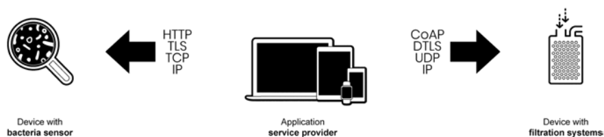
Figure 13.2 Example of Device-to-Cloud communication. Bacteria sensor and filtration system with built-in cloud-connection. Adapted from Tschofenig et al. (2015).
