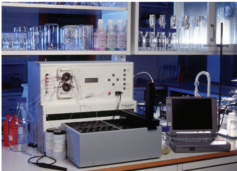
Figure 6.2 The first semi-automated Colifast laboratory analyser: CA 100.
