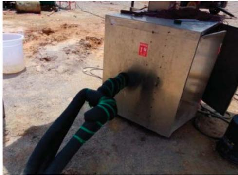
Figure 4. Thermal response tester.
