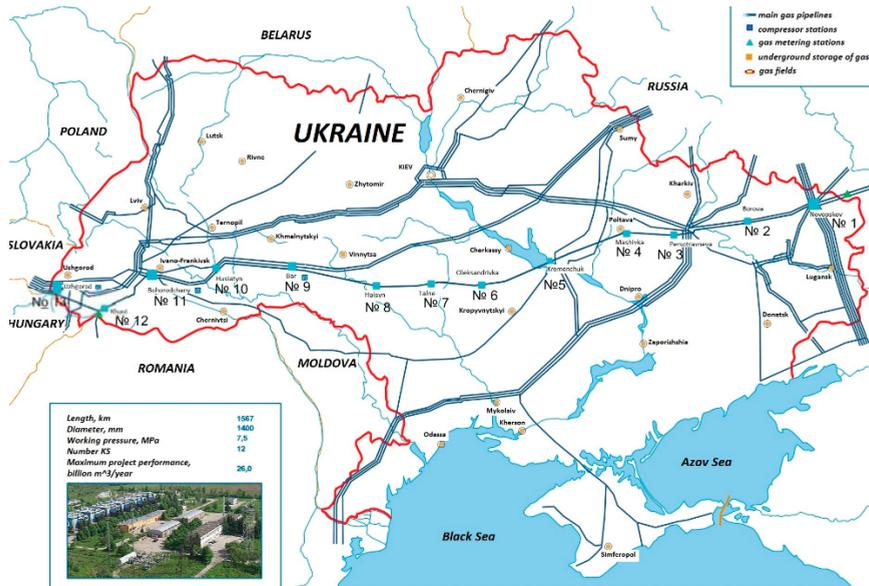
**Figure 4.** The GTS of Ukraine with the designated “Soyuz” gas main with a total length of 1567.3 km (the territory of Ukraine), a diameter of 1420 mm, and a wall thickness of 20 mm, which has 13 compressor stations (CS) equipped with GTK-10I gas-pumping units along its route: 1. Novopskov; 2. Borova; 3. Pershotravneva; 4. Mashivka; 5. Kremenchuk; 6. Oleksandrivka; 7. Talne; 8. Haisyn; 9. Bar; 10. Husiatyn; 11. Bogorodchany; 12. Khust; 13. Uzhgorod.
