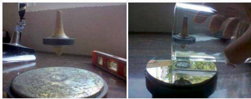
Figure 6. Magnetic levitation by fast rotating magnet.
