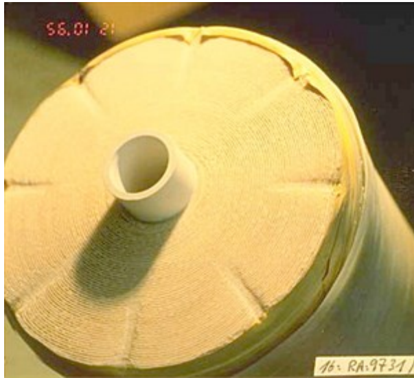
Figure 59. The endcap has been pushed off
