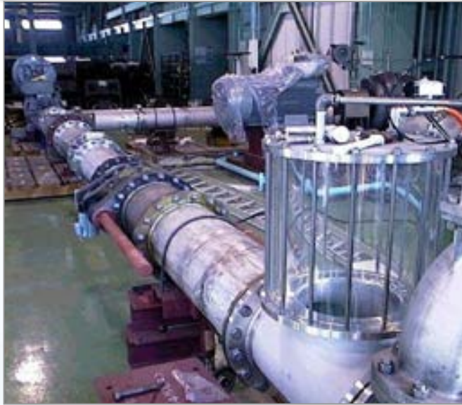
High Specific Speed (Ns) Pump Test Loop
