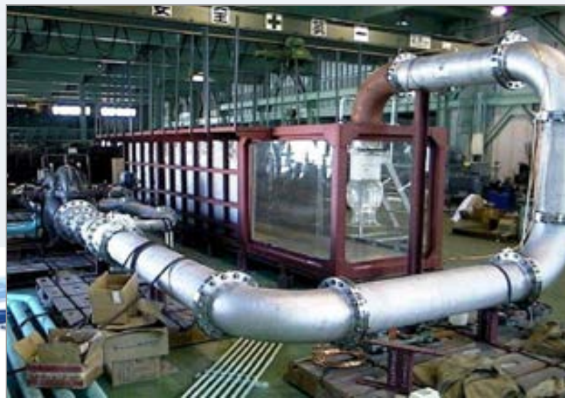
High Specific Speed (Ns) Pump Test Loop
