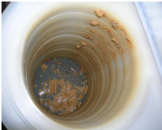
Figure 3-4: Scale formation at the cassette entrances
