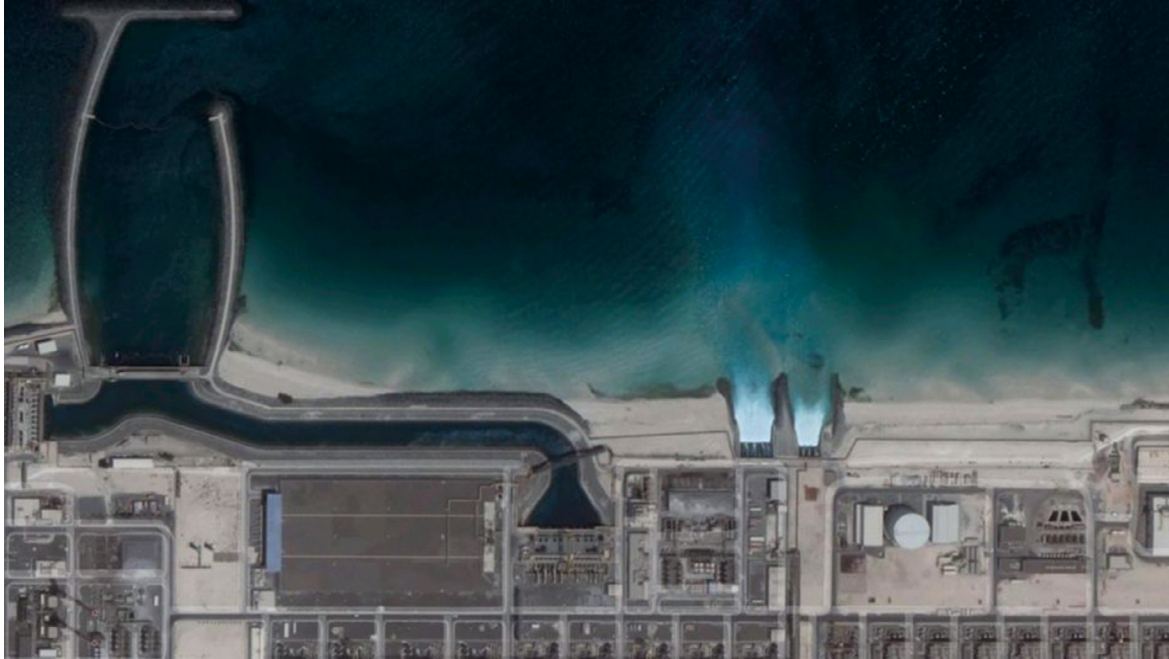
Figure 6: Jebel Ali MSF plant, UAE, power and water cogeneration plant, positively buoyant discharge
