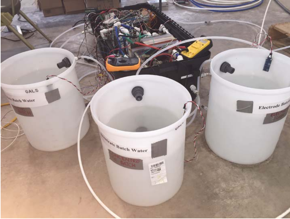
Figure 30. Batch tanks: dilute, concentrate, electrode flush.
