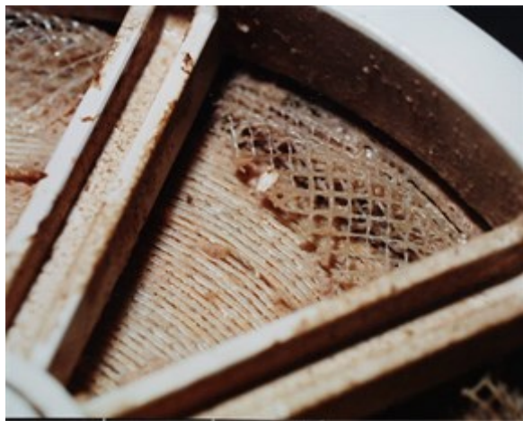
Figure 60. High pressure drop due to biofouling has pushed out the feed spacer
