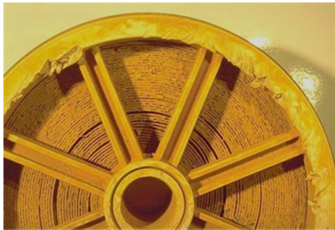
Figure 56. Picture of iron fouled feed side of an element with telescoping damage and signs of mechanical force
