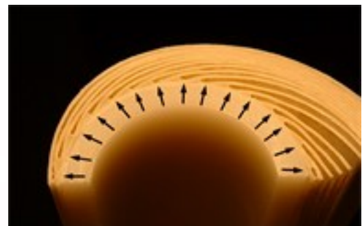
Figure 14. Cross-section of a permeate water tube through the side glue lines of the leaves
