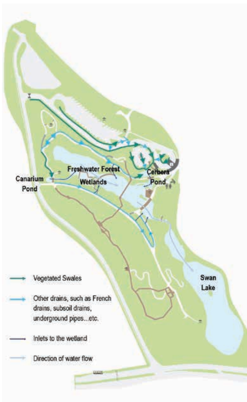
Fig. 10.19 The water treatment system at the 10-Hectare Learning Forest
