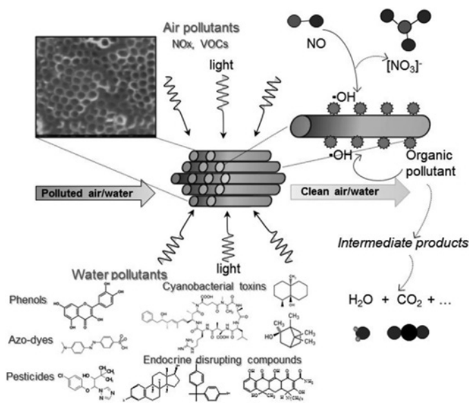
Figure 8.3 Photocatalytic purification of air and water pollutants flowing through tubular TiO 2 nanostructures.
