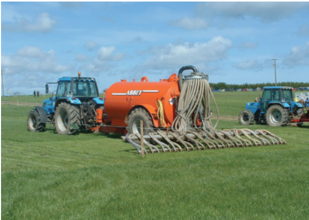
Figure 1.2: Slurry tanker having a system of trailing shoe applications made by Craggs et al. (2004), and could be a substitute on dairy farms.
