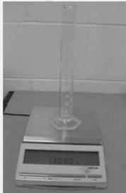
Place 100 mL graduated cylinder on a scale
