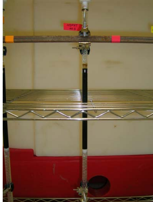
Figure 2.1 Schematic of a typical set up for a column study
