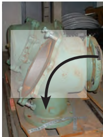
SUCTION DIFFUSER STRAINER The screen occupies the area indicated by the shading. Flow is as indicated by the arrow.
