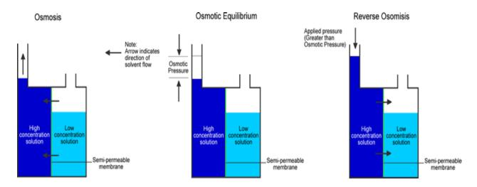
The desalinated water that is de-mineralized or de-ionized, is called permeate (or product) water. The water stream that carries the concentrated contaminants that did not pass through the RO membrane is called the reject (or concentrate) stream. From the data collected from Reverse Osmosis System manufacturers, normally 40-60% water is rejected during the Reverse Osmosis process.
