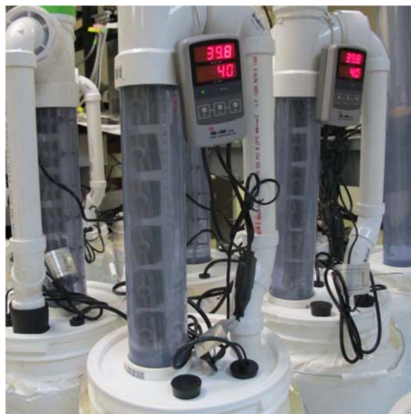
Figure 4.15 Test vessels, schematic on left and photo of exposure column on right
