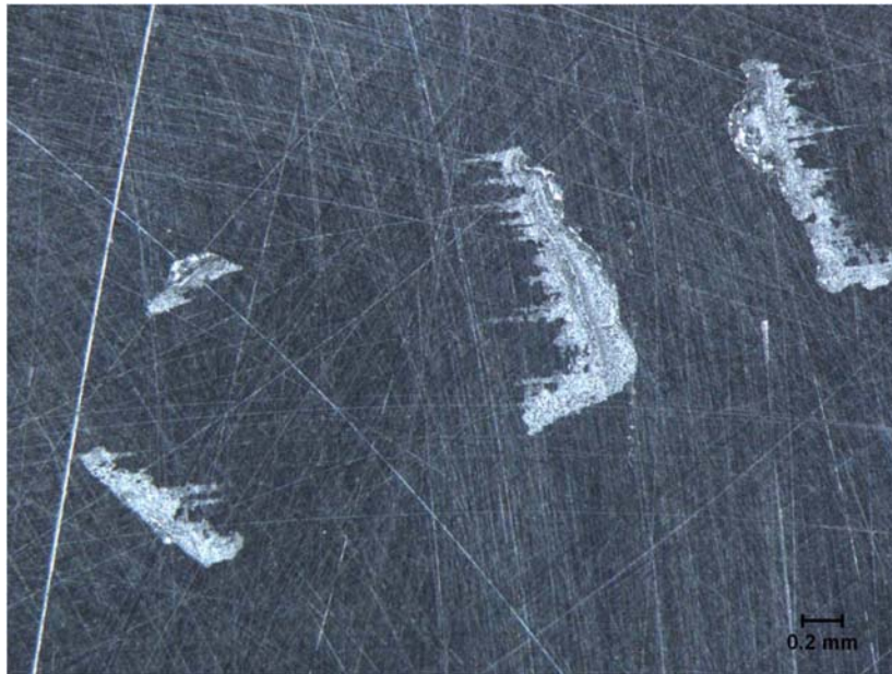
Figure 4.9 Close-up of crevice corrosion on Alloy 2205, 25X magnification
