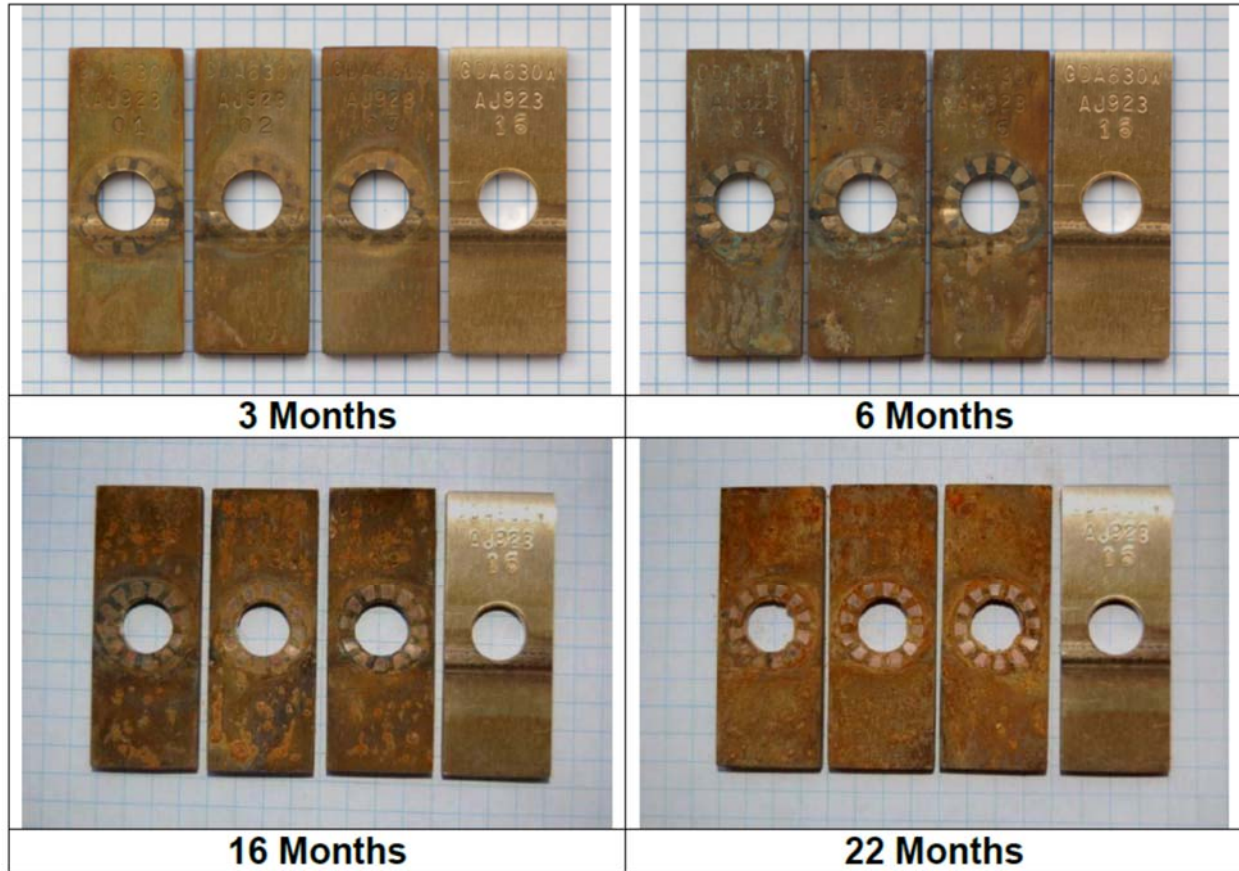
Figure 3.27 Corrosion progressions in the CDA630 alloy coupons
