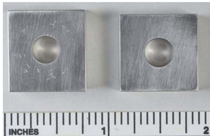
Figure 4.5 Specimen AQR2 (left, 316L) and AVM16 (right, 2205) after exposure to 10,000 mg/L chloride, no free chlorine, pH 5, at 30°C. Crevice corrosion is present in lighter areas
