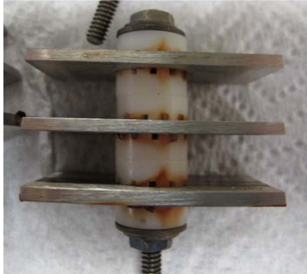
Figure 4.16 Test specimen assembly consisting of 316L SS specimens after 90 days of exposure; Note rust stains on crevice washers
