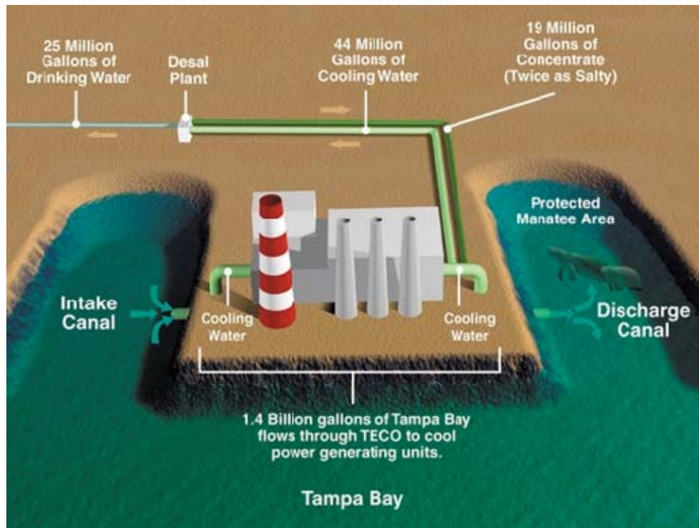
Figure 7 – Tampa Bay SWRO Plant Collocation Schematic
