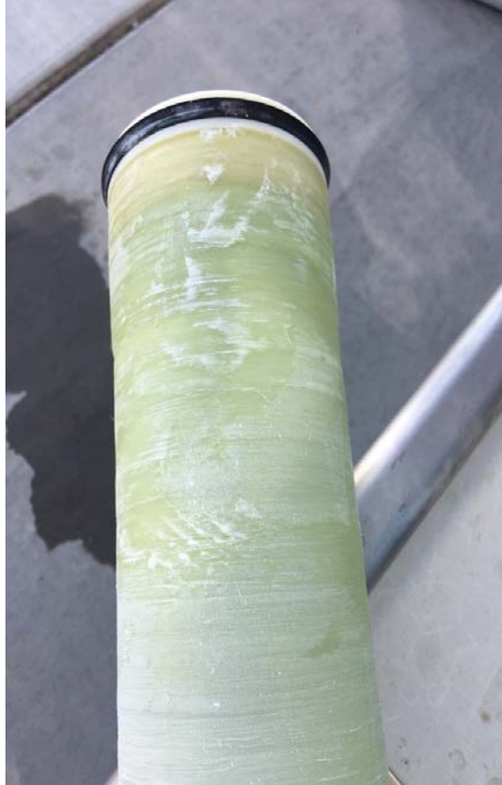
Figure 28. Observed scaling on outside of CRRO tail element prior to autopsy.
