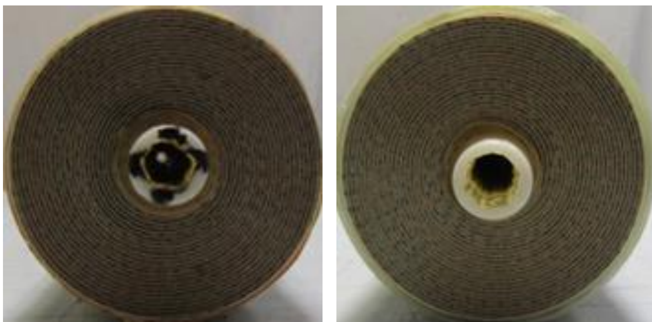
Image of feed scroll end (left) and concentrate scroll end (right) for SN# 11518561
