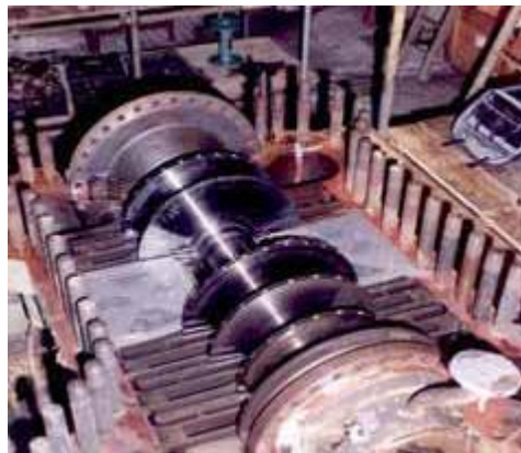
Fig.8. Barrel type multistage centrifugal compressor
