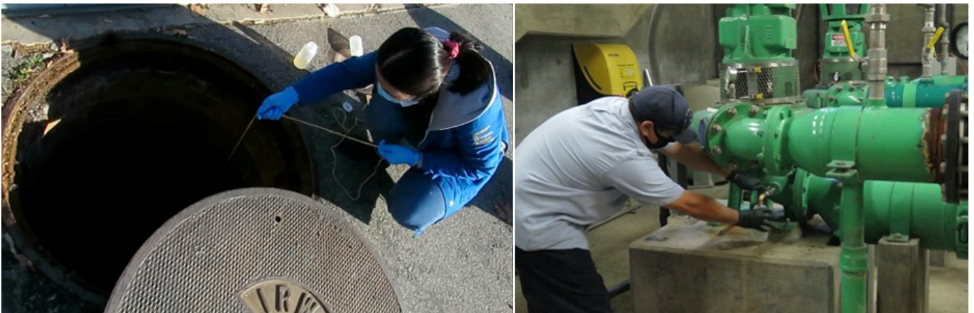
Images of a sampling event at the lift station influent (left) and effluent (right)
