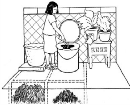
Double Vault urine diverting dry eco-toilet
