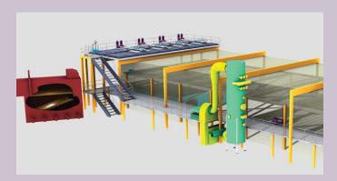
**BioCon™ ERS** (Energy Recovery System) is a safe and sustainable drying and combustion system that combines the efficiencies of a convective air low temperature belt dryer with a biomass furnace to recover sensible heat and combust all organic material.
