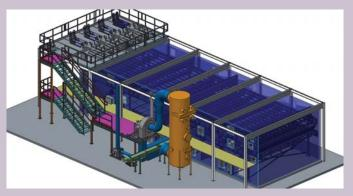
The low temperature nature of the thermal sludge dryer enables the BioCon™ dryer to utilize various thermal energy sources including thermal oil, air or steam. Thermal efficiency can be further increased by employing BioCon™ Energy Exchange System. Fuel sources for the Biocon™ system include natural gas, biogas, or fuel oil.
