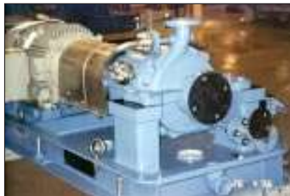
Photo 2. Example of an API process pump
