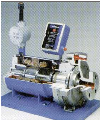
Cutaway view of a canned motor pump. These pumps are used on a wide variety of fluids at temperatures from cryogenic service to 1000° F and at system pressures up to 5,000 PSI.
