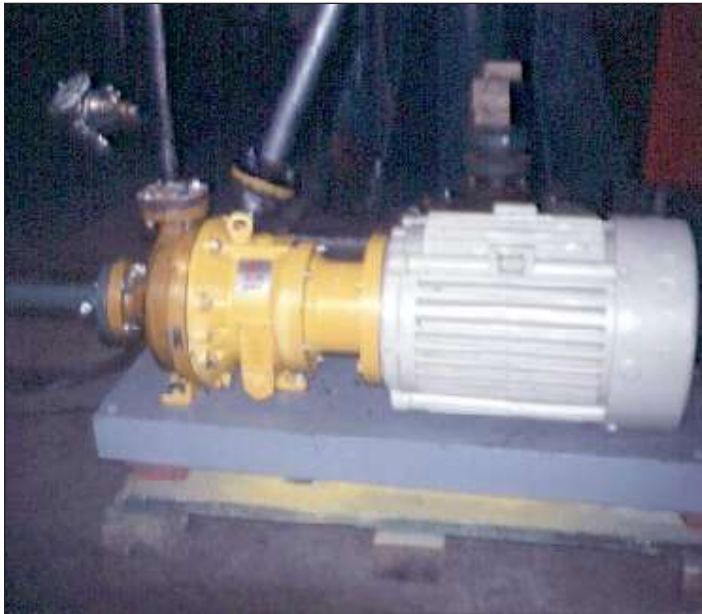
An A range pump hooked up for testing.
