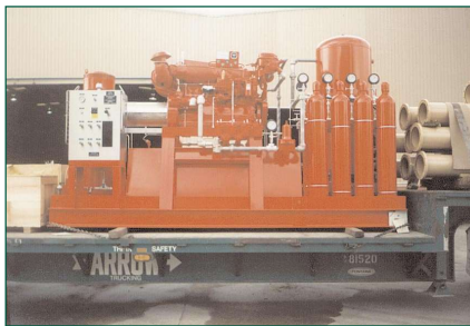
Photo 3. Vertical fire water pump for offshore installation. Compressed air start with back-up nitrogen system and expansion receiver
