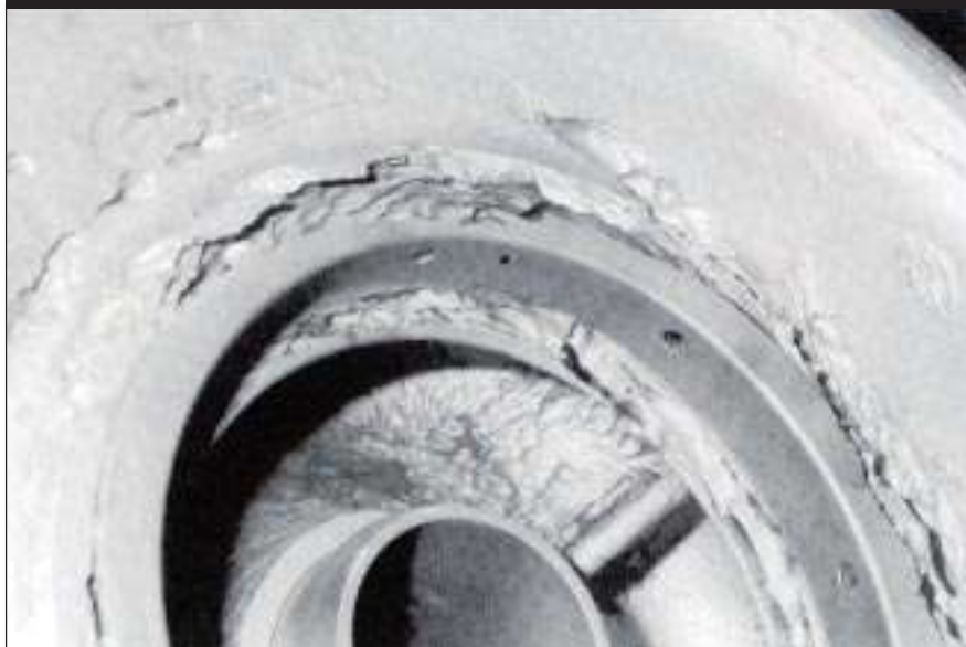
Conventional API process pump internals can be destroyed in a matter of days during prolonged upset operating conditions.
