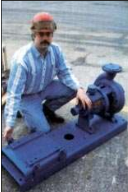
Photo 1. Recently received group two size pump incorporates motor jacking bolts, grout hole, bearing isolators, bull's eye oil indicator and bearing housing expansion chamber as standard features.
