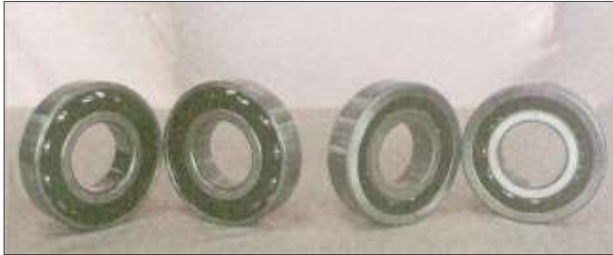
Photo 2. Two pairs of DACBs, with the pair on the left positioned face-to-face, the pair on the right back-to-back
