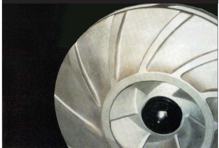
Enclosed impeller with front and back repelling vanes to reduce circulation of the slurry.
