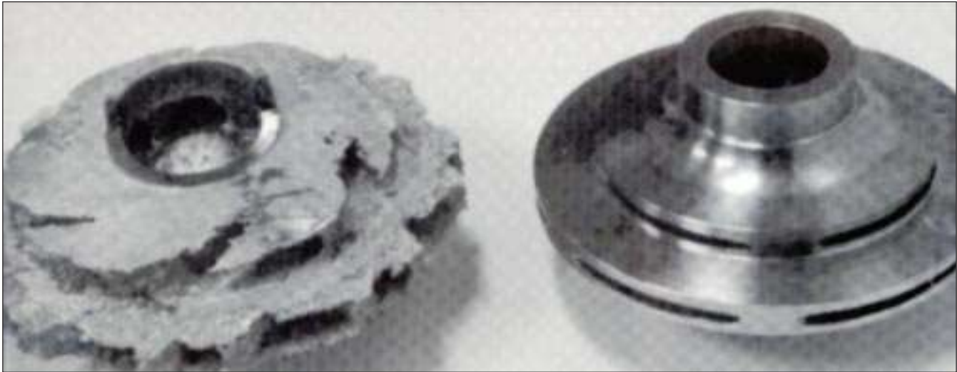
Photo 1. New and corroded centrifugal pump impellers.
