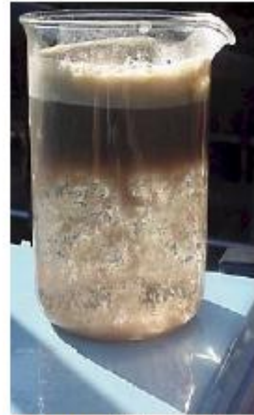
1) Meat Rendering Water Processed With The Elgressy Electrocoagulation System
