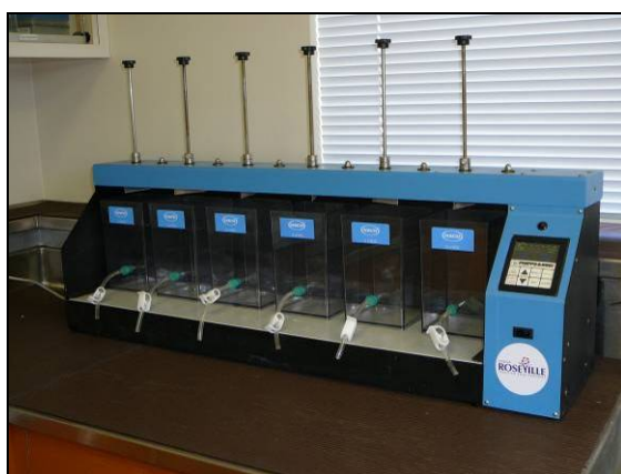
Figure 19: Wagner™ Jar with Phipps Bird multiple stirrer
