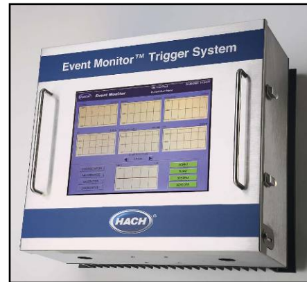
Figure 13: Source Water Panel and the Event Monitor® Trigger System The Source Water Monitoring Panel can be configured with six probes selected to meet the particular needs of the individual water source. Select from the Solitax, pH, conductivity, ORP, LDO, NH4D, NitraTax and UVAS. Combine the panel with a TOC Analyzer and the Event Monitor for the most sophisticated source water monitoring system available. Hach Company stock photos
