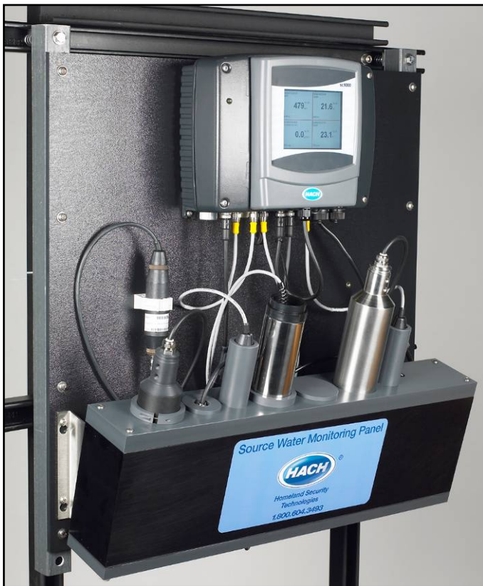
Figure 13: Source Water Panel and the Event Monitor® Trigger System The Source Water Monitoring Panel can be configured with six probes selected to meet the particular needs of the individual water source. Select from the Solitax, pH, conductivity, ORP, LDO, NH4D, NitraTax and UVAS. Combine the panel with a TOC Analyzer and the Event Monitor for the most sophisticated source water monitoring system available. Hach Company stock photos
