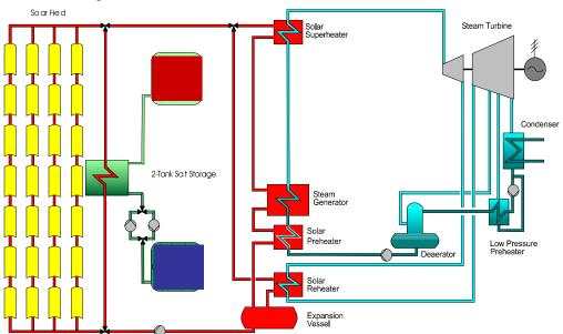
Figure 4: Parabolic trough system schematic
