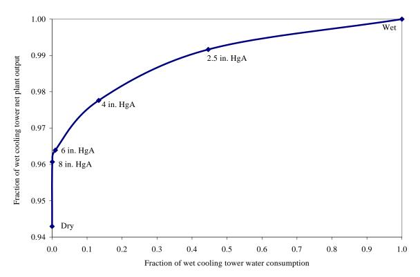
Figure 6 Net Plant Output as a Function of Wet Cooling Tower Water Consumption
