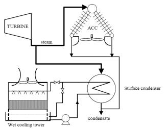
Figure 11: Hybrid wet/dry parallel cooling system (PCS)
