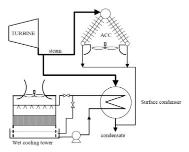
Figure 3 Schematic Diagram of Hybrid Heat Rejection System
