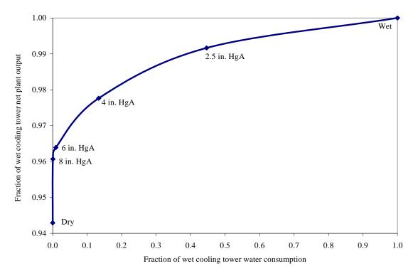
Figure 12: Power plant output as a fraction of the output for an evaporatively cooled plant vs. the fraction of water consumed.
