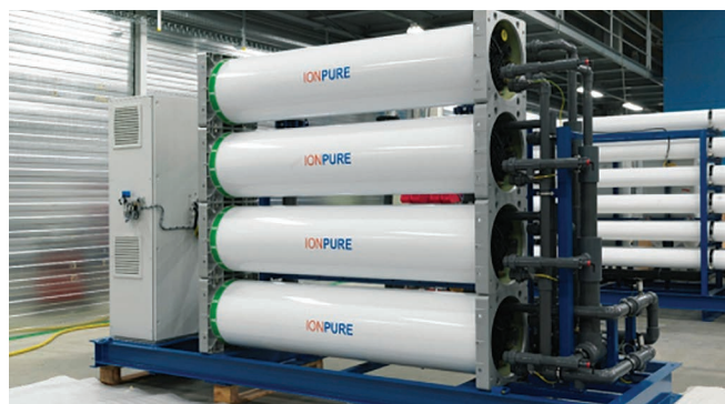
Figure 4 264 gpm (60 m³/h) CEDI system using stacked-disk modules
