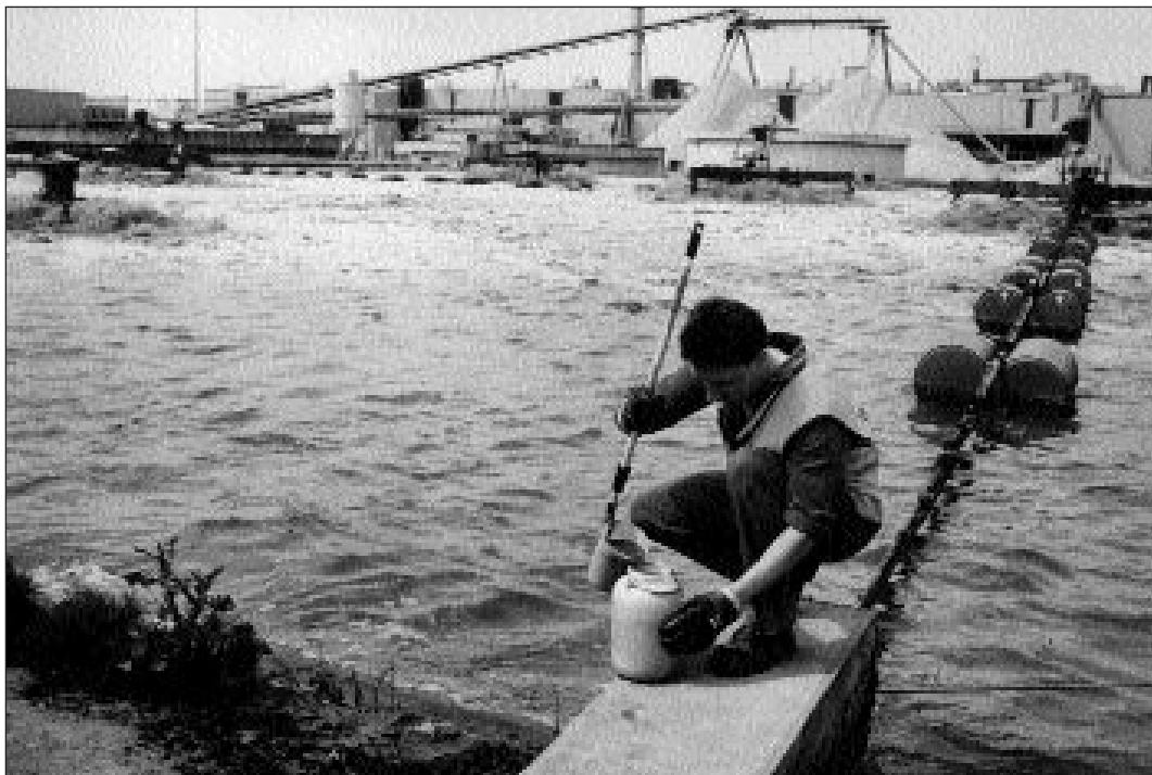
Sampling from the aeration lagoon
