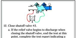
failed device and that check valve #1 is leaking.
