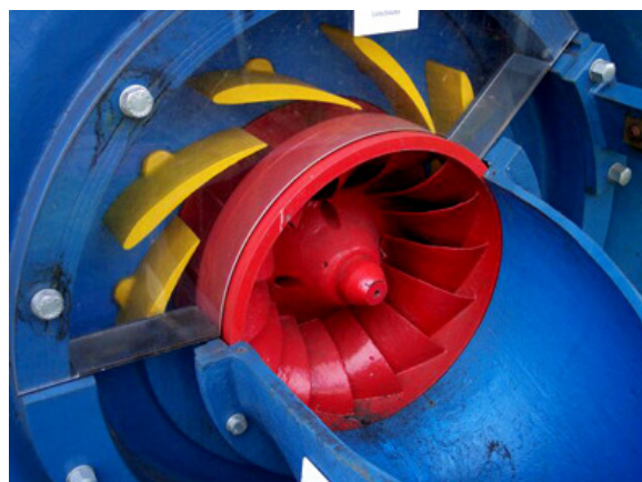
Figure 10: Horizontal axis Francis turbine
