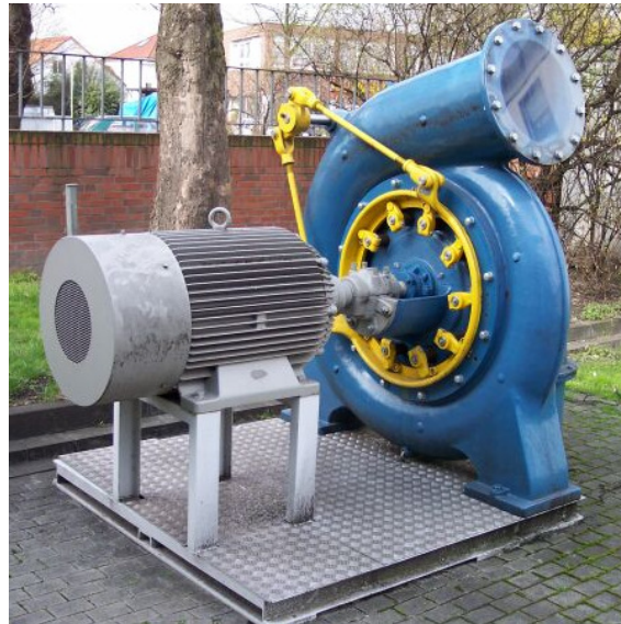
Figure 9: Francis turbine with generator (Guirguis, 2011)
