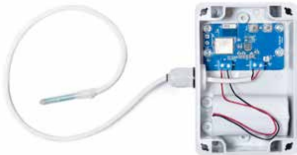
Figure vi. Dropula Smart Water Meter
