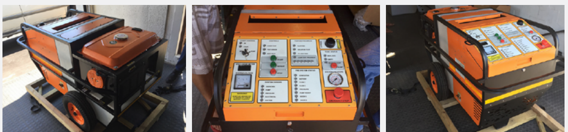
Figure v. The Pipe Condition Assessment Device
