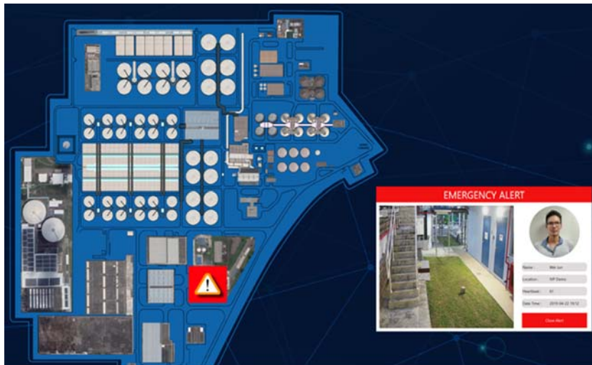
Figure 3.10 Geo-fencing intruder alert system.
