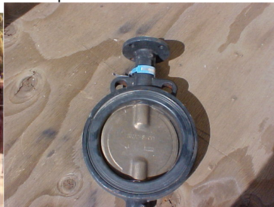
Large Gate Valve and a Butterfly Valve which works like an old fashioned carburetor.
