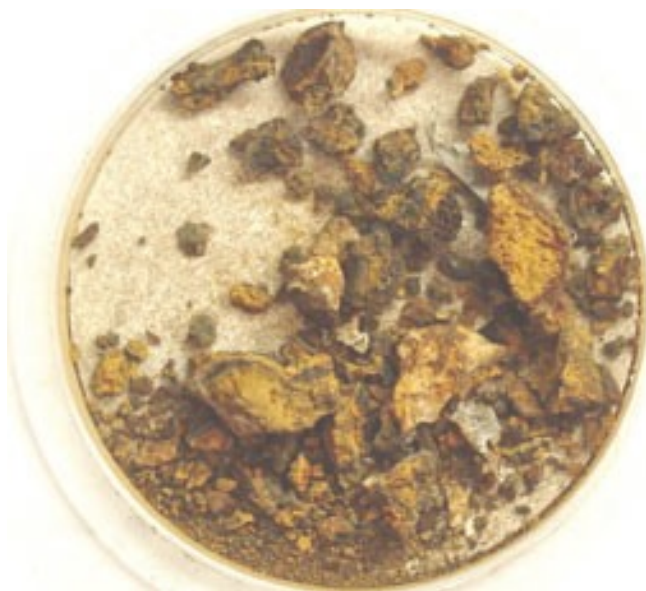
Large Rust Particles
