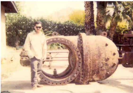
Large Gate Valve and a Butterfly Valve which works like an old fashioned carburetor.
