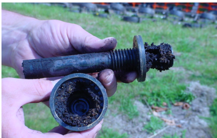
Figure 5.13: Example of blocked nozzle.
