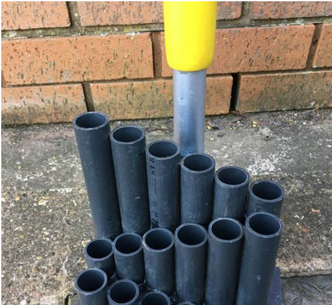
Figure 5.16: Backwash expansion measurement tool is shown
