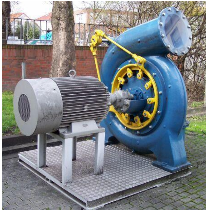
Figure 2-1: Francis Turbine with Generator
