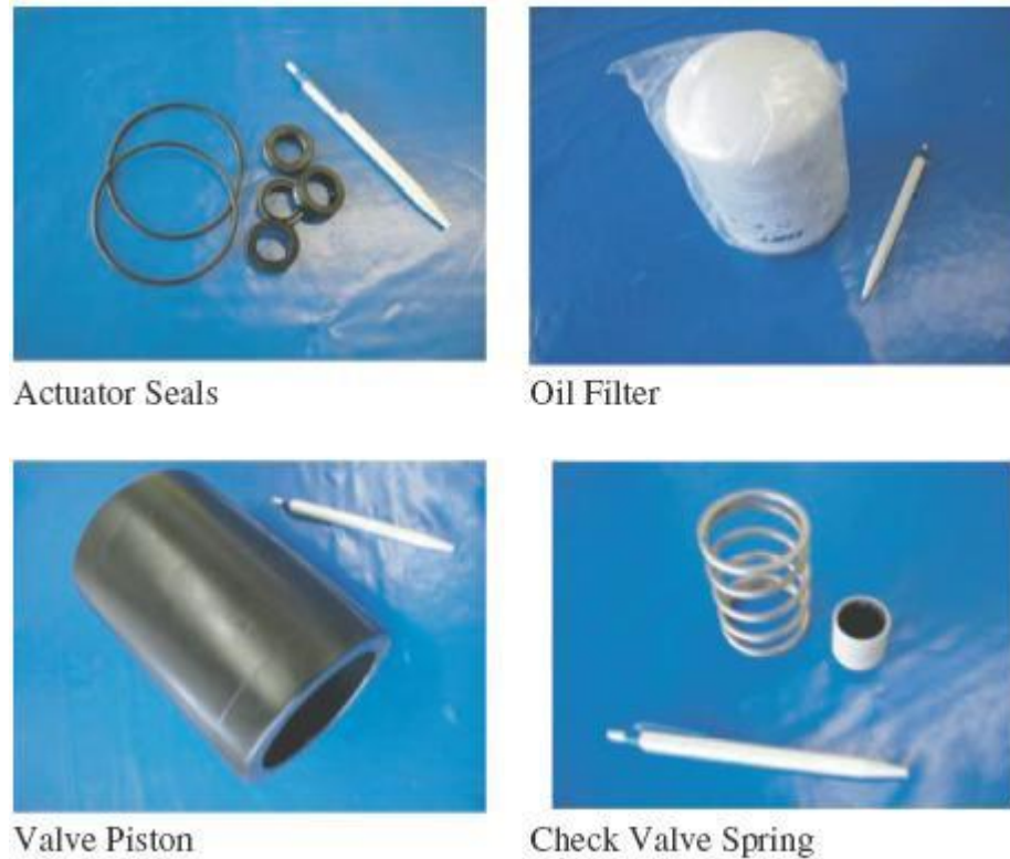
Figure 6-8: Wearing Parts Which are to be Changed
