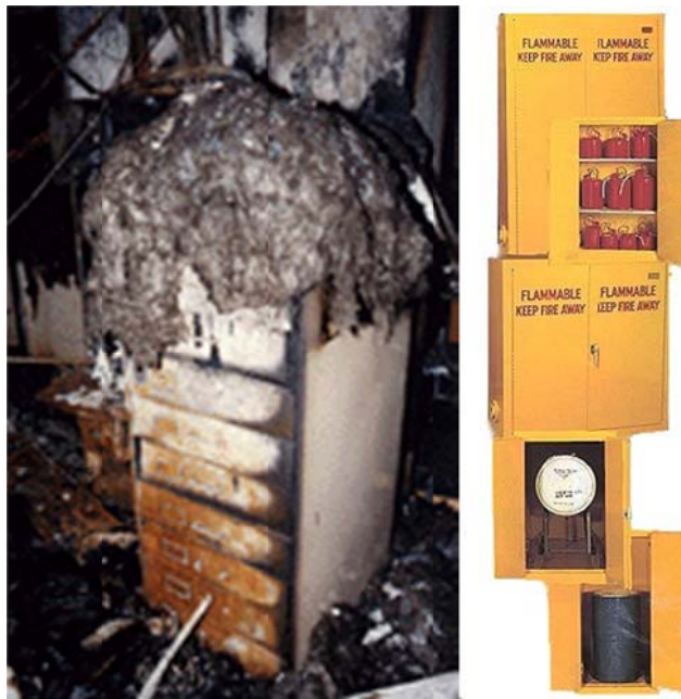
A fire resistant file cabinet that is burned completely and beside it are modern flammable liquids storage cabinets.
