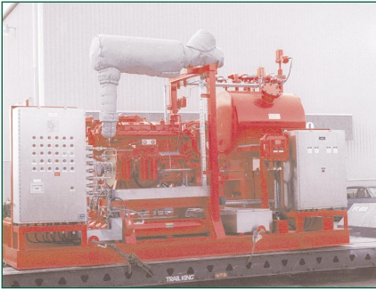
Photo 2. Custom fire water pump system designed for Class 1, Groups C & D and Division II. The controller features all NEMA 7 switches mounted in a stainless steel cabinet. The battery charger and battery case are purged and constructed of 316SS. The system has a primary electric start with a back-up hydraulic system.
