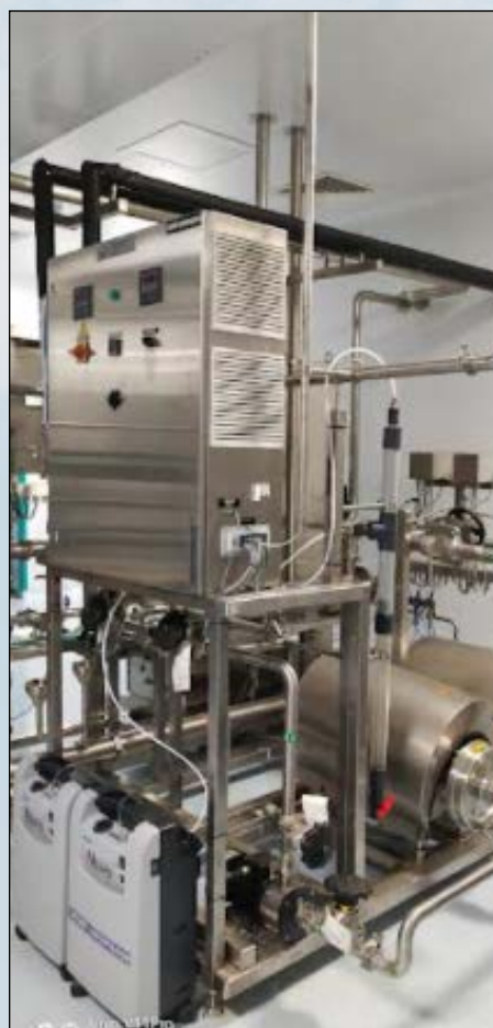
Ozone System using small oxygen Concentrators
