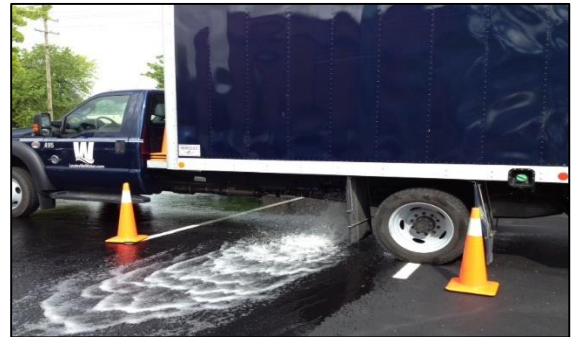
Figure 7 Meter testing via truck mounted apparatus
