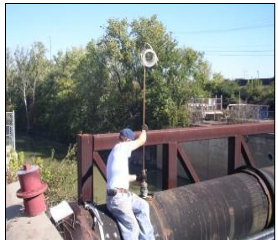
Figure 8 Pitot rod inserted into large pipeline
