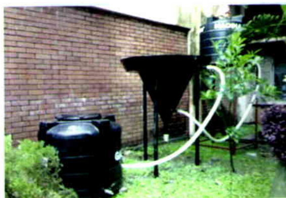
Figure 4.32 : ARUBA Arsenic Removal Plant Prototype
