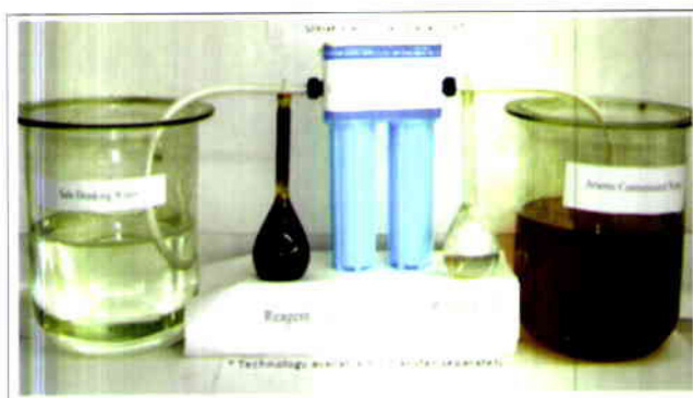
Figure 4.31: Ultrafiltration Membrane Assisted Process
