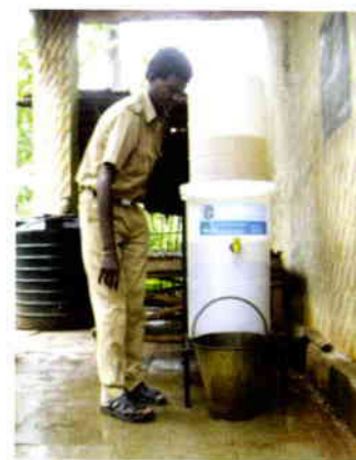
Figure 5.3: Household Iron Removal - CSIR - NEERI Technology
