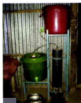
Arsenic removal 'Family Filter'
