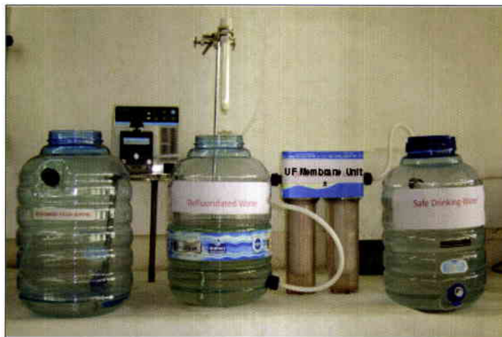
Figure 3.15 : BARC Defluoridation Unit
