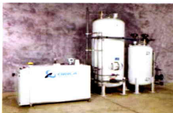
Figure 6.4: MIEX® Treatment Systems
