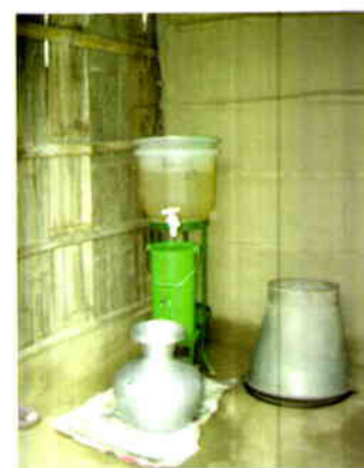
Figure 4.14: Read-F Arsenic Removal Unit
