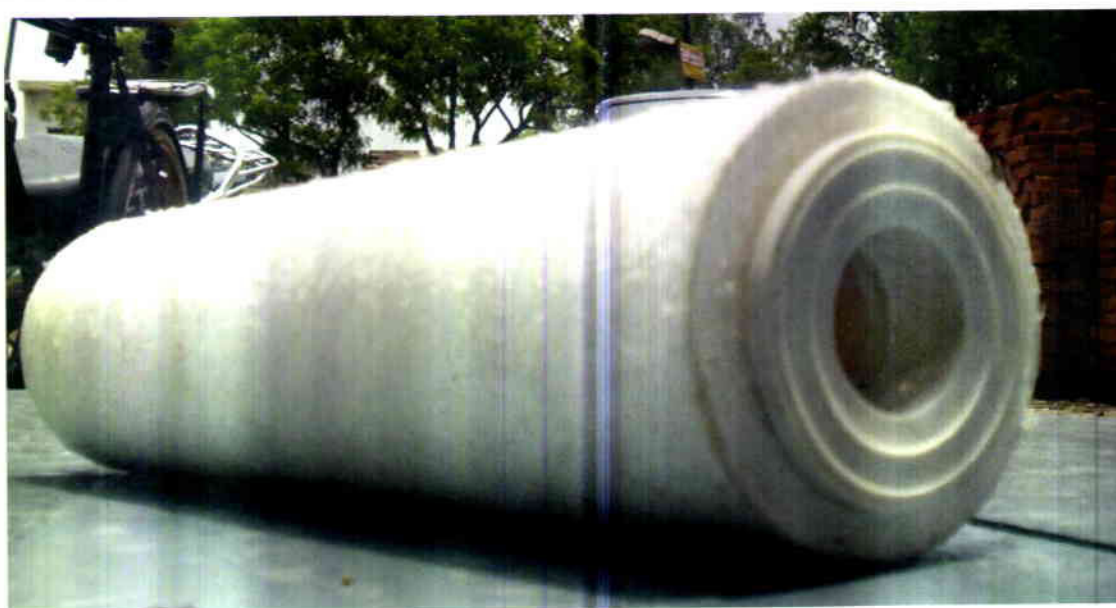
A view with netted top Polypropylene Filter
