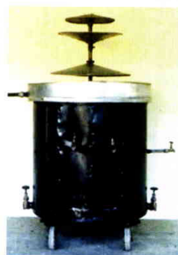
Figure 5.7: Water Iron Removal Unit of DRDO
