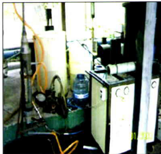
Figure 5.11: UF Membrane Assisted Device for Removal Of Iron
