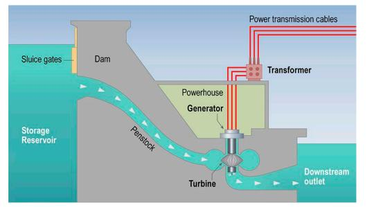
Figure 8-6. Cross section of a large hydroelectric plant
