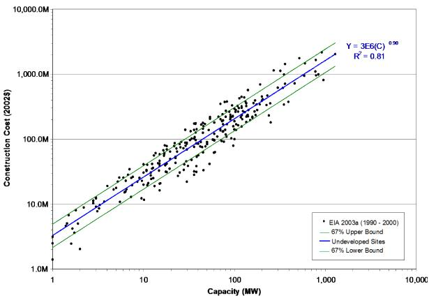
Figure 8-10. Original construction cost-estimating curve (2002\$) Source: Idaho National Laboratory
