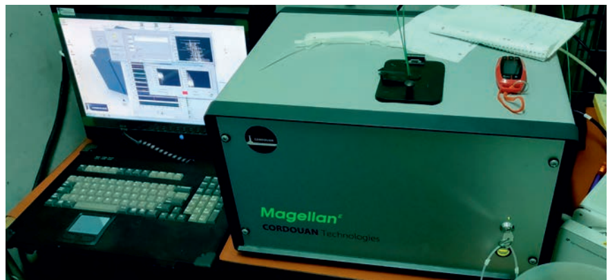
Figure 1: The laser-induced breakdown-detection (LIBD) device set up in the Kranji NEWater Factory (KNF).
