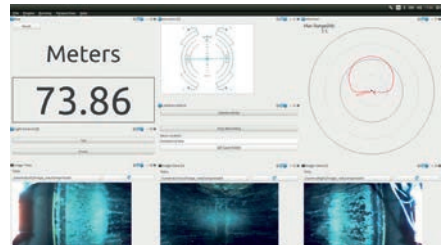
Figure 2: The front pan-tilt-zoom (PTZ) camera view (left) and the user interface with three images from the robot's inspection array (right).
