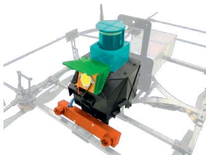
Figure 1: The design of the multi-sensory unmanned aerial vehicle (UAV).
