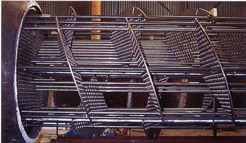
Helix Heat Exchanger Tube Bundle in Fabrication
