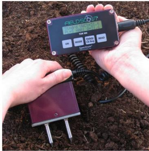
Fig. 24.5. TDR probe for soil water measurement.
